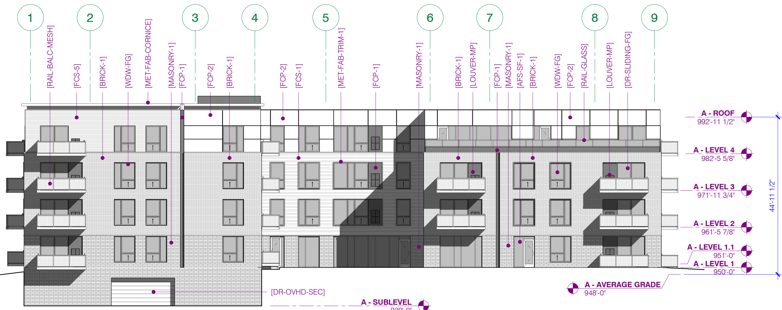
3 A - EXTERIOR ELEVATION SOUTH
