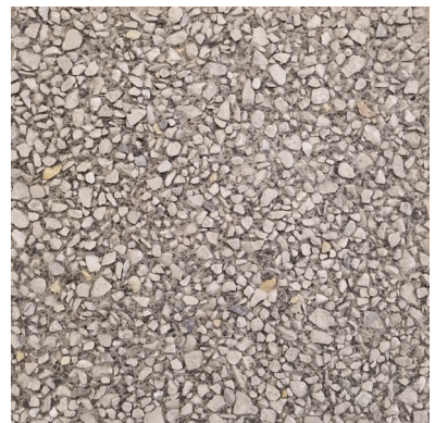
PRECAST CONCRETE PANEL LIGHT GRAY EXPOSED AGGREGATE (MATCH EXISTING INGOT FACILITY)
