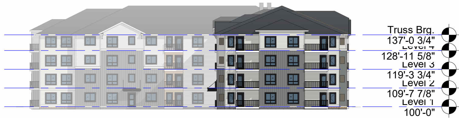
3 Building A - East Elevation 1" = 30'-0"
