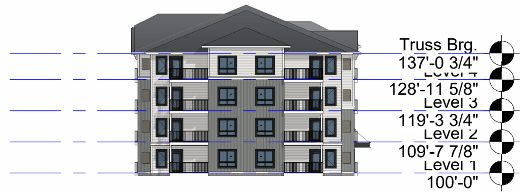
2 Building B - North Elevation 1" = 30'-0"
