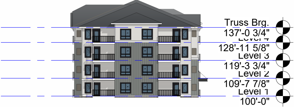
2 Building B - North Elevation 1" = 30'-0"
