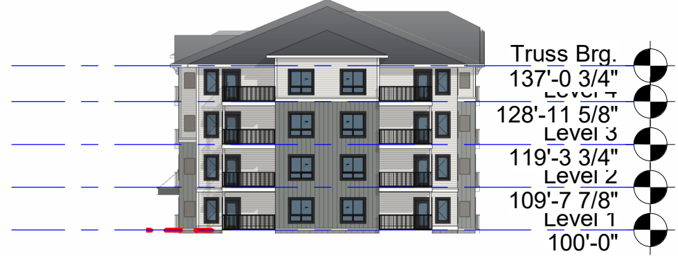
3 Building B - South Elevation 1" = 30'-0"
