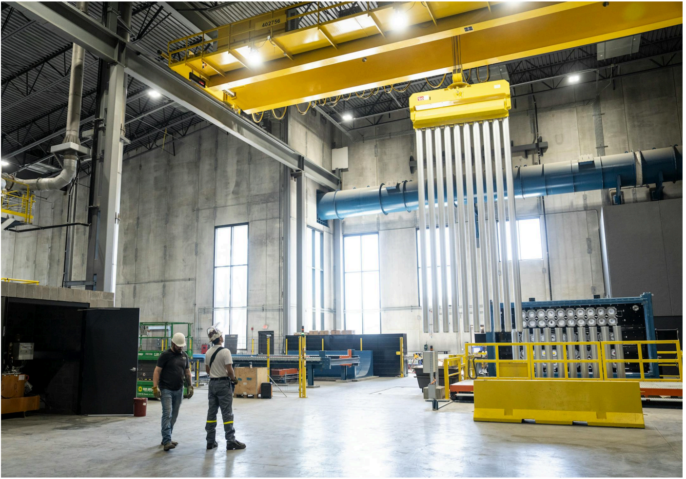
Lorenzo Martinez, right, uses a remote control to guide hanging 24-foot recycled aluminum billets at Spectro Alloys in Rosemount. (Renée Jones Schneider/The Minnesota Star Tribune)
